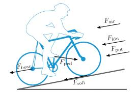
The equilibrium of forces is given by a differential equation with the parameters in the table which must be measured or taken from the literature.
