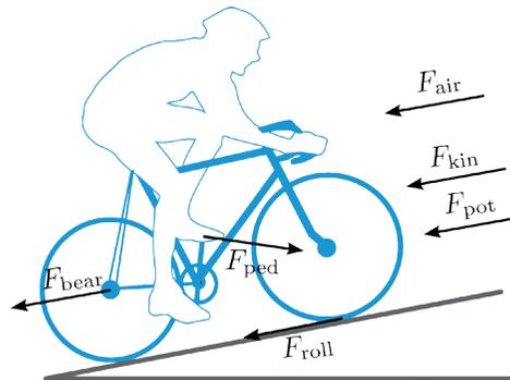
The equilibrium of forces is given by a differential equation with the parameters in the table which must be measured or taken from the literature.
